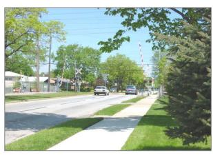
Figure 3-14: Looking north across the Crawford Avenue grade crossing. The typical elements of the warning equipment (auto and pedestrian gates), flashers, etc., are visible. Note the residential nature of the surrounding neighborhood.
