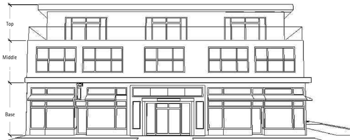
Articulated building with clearly defined base, middle and top.
