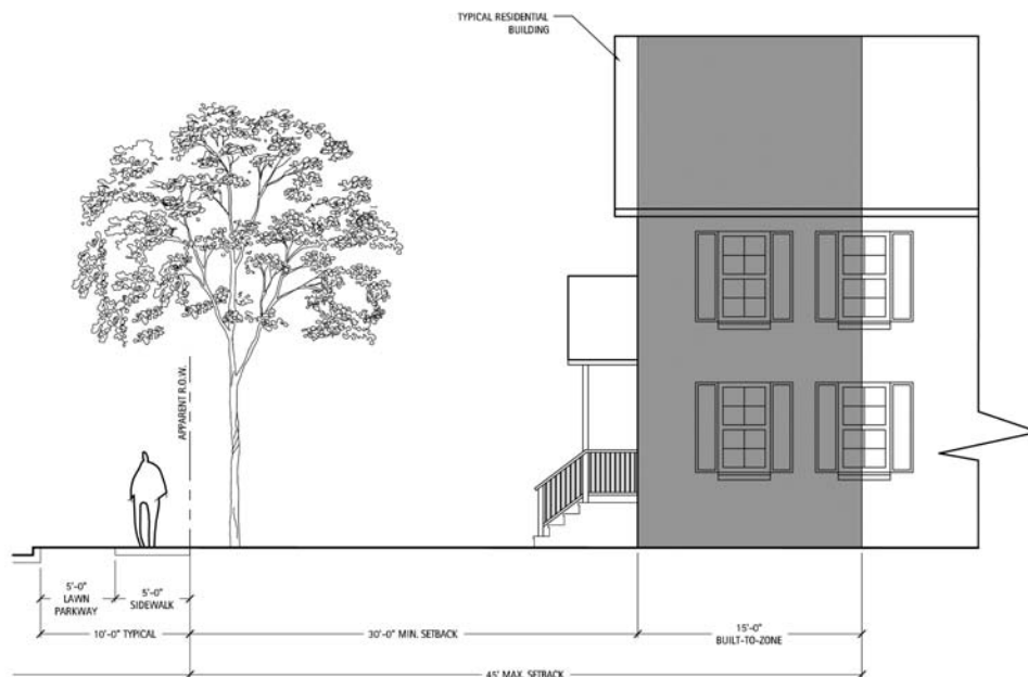
Figure 3.24: Typical Section in MT District
