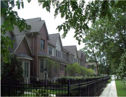
Varied rooflines and bay windows break down the overall mass of this row of townhouses.
