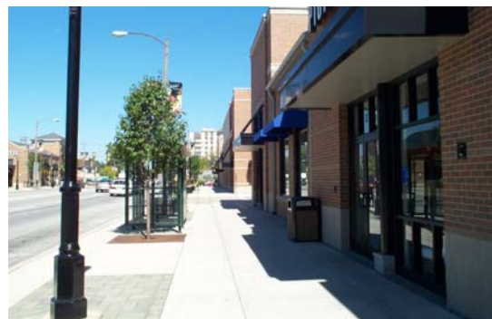
A generous sidewalk width allows for both a walking zone and an amenity zone to accommodate light poles, street trees, bus stop shelters and other streetscape features.
