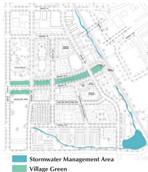
Figure 29: Phase 2 Open Space and Stormwater Management Area
