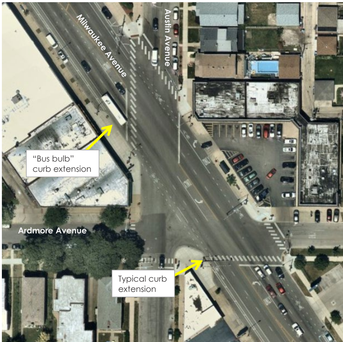
Figure 20 – Aerial view showing two example curb extensions, one of which includes a bus stop. Source: Nearmap, 2017.
