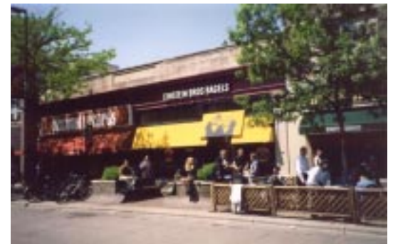
These simple pitched fabric awnings protect against the sun and provide visual interest. Facade-width awnings are appropriate here because the store consists essentially of one wide bay.
