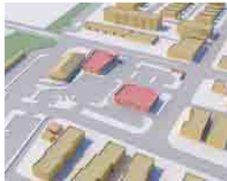
Dempster access to parking areas. Drive-through layout avoids back-up of vehicles into the parking lot or street.
