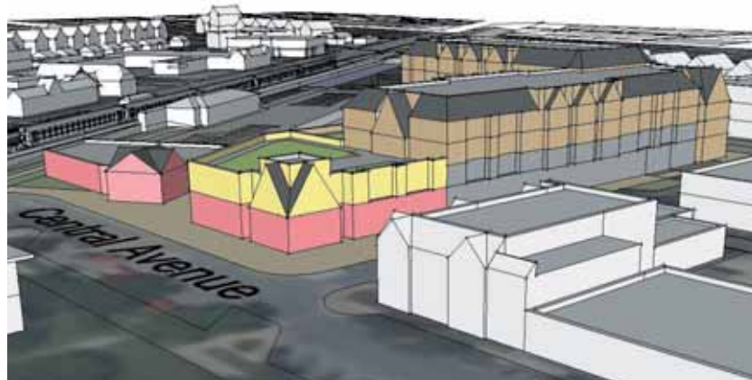
Conceptual three-dimensional building and site massing study for the Chase Bank/UP Site shows the idea of creating a continuous “street wall” along Central Avenue.
