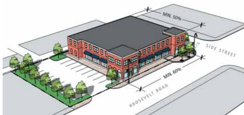
Example form-based code graphic that emphasizes building, site and parking design and relationships.
