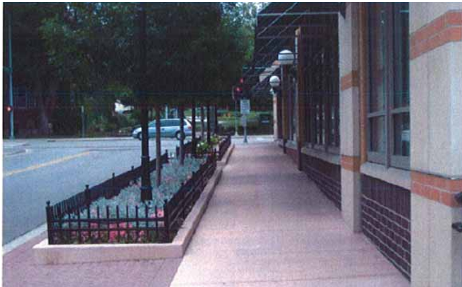
Six-foot wide planting strip with vertical curb to provide buffer and facilitate landscaping with street trees. Source: Smart Transportation Guidebook, 2008. New Jersey Department of Transportation/ Pennsylvania Department of Transportation.
