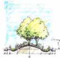
Detail 1 - Cross section showing a wide section of the median with two bioswales
