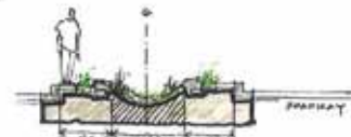
Detail 2 - Cross section showing a narrow section of the median with one bioswale
