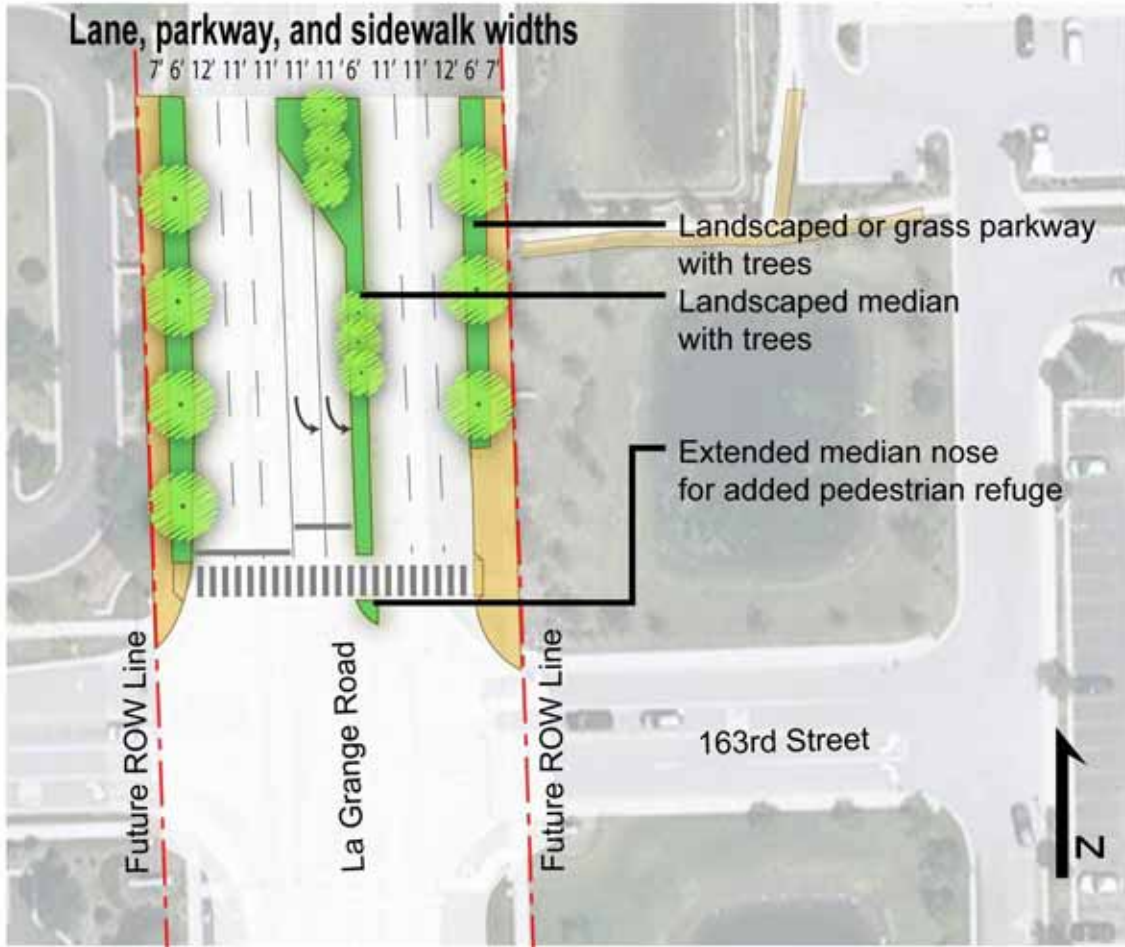
Conceptual sketch of La Grange Road at 163 rd Street showing lanes reconfigured to facilitate wider parkway treatments and improved pedestrian facilities.
