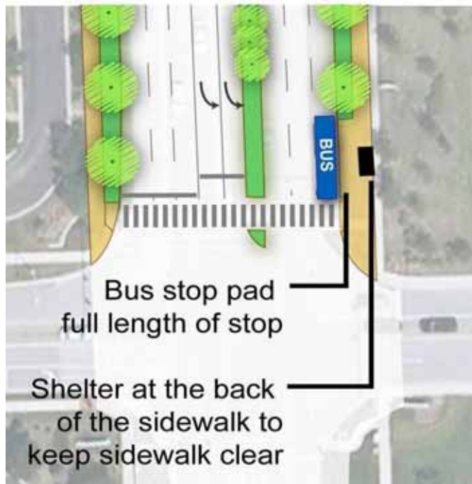
Concept sketch showing the typical preferred location of a far side bus stop on La Grange Road.
